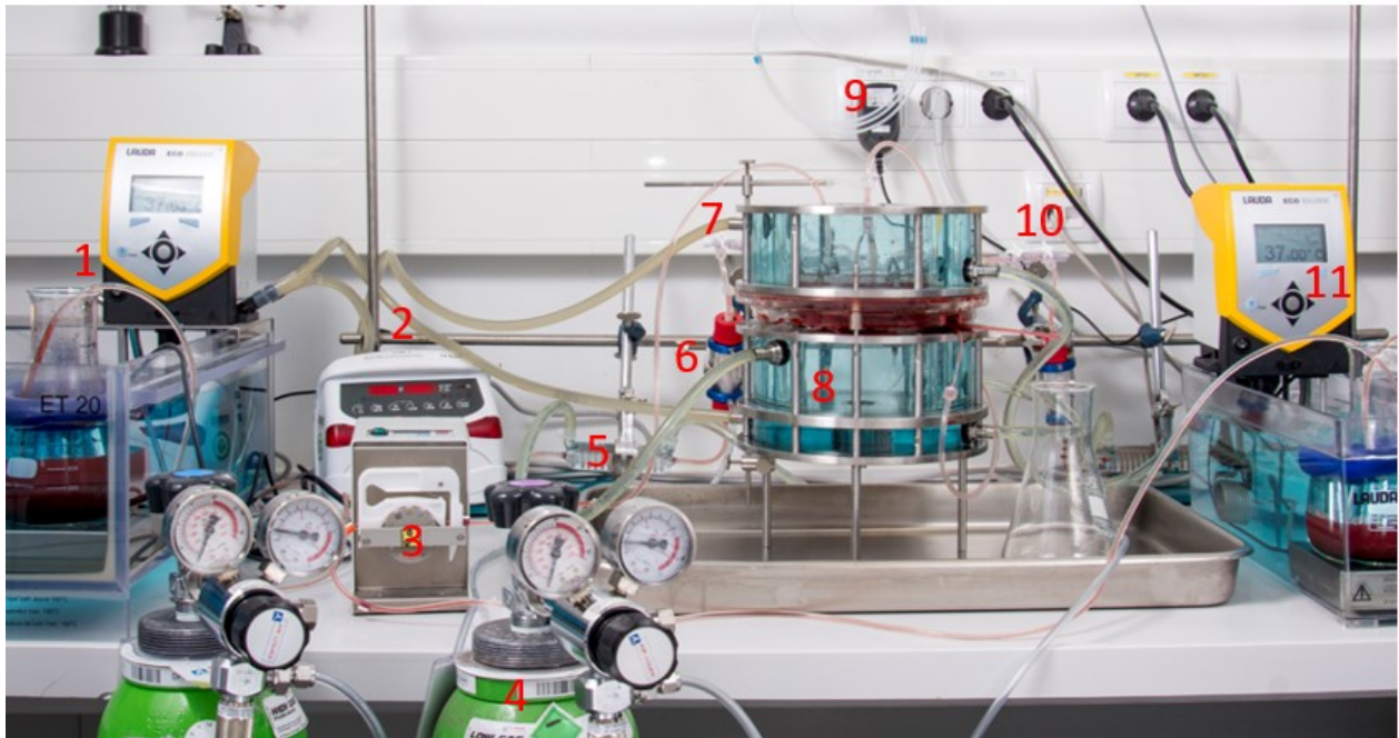
Figure 6. Ex vivo placental perfusion setting as used for this thesis. 1) foetal reservoir 2) pump for foetal circulation 3) pump for maternal backflow 4) perfusion gases 5) glass heat exchange coil 6) gas exchange membrane 7) foetal arterial sampling port 8) perfusion chamber 9) pressure sensor catheter 10) maternal arterial sampling port 11) maternal reservoir
