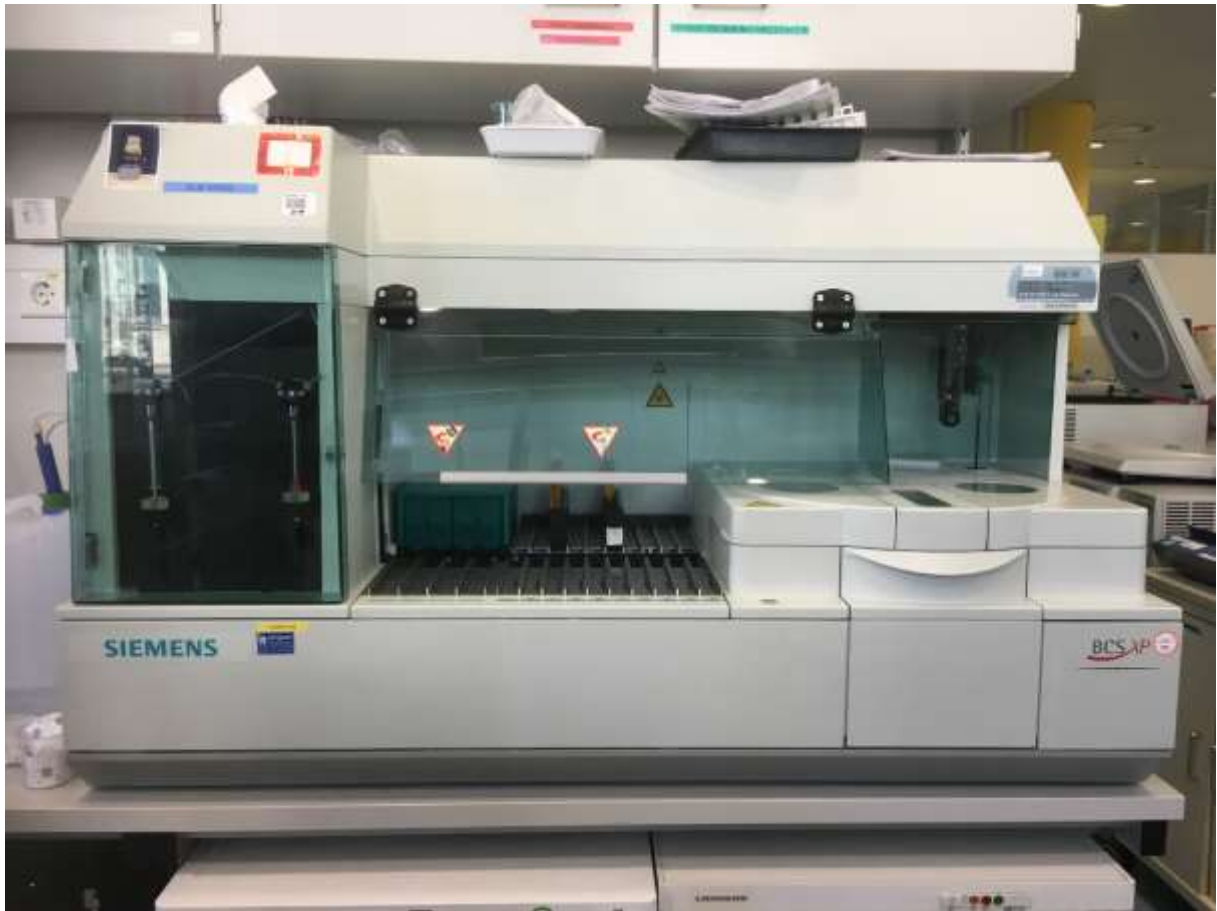
Fig. 7. BCS XP coagulation analyzer (Siemens Healthcare Laboratory Diagnostics, Tarrytown, NY, USA) (image source: Sarah Niessner)
