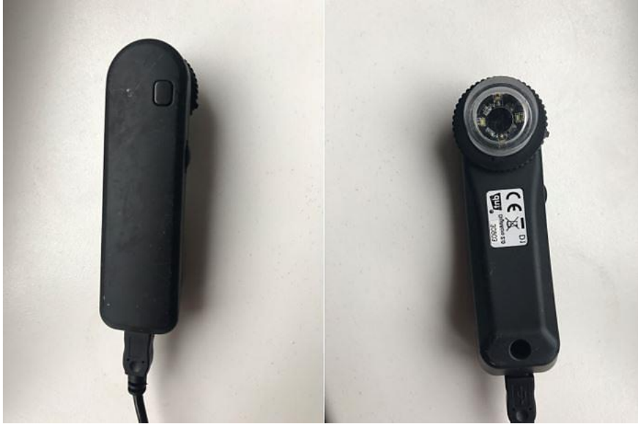
Figure 16. Macroscopic images of the reference areas were taken with a special microscope camera.
