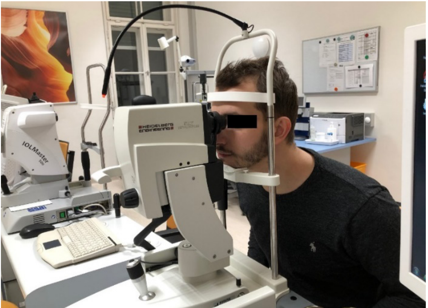
Figure 3. Spectral domain optical coherence tomography. (University Eye Clinic, Graz, 16.11.2018) The study subject focuses on a blue dot in the device while the images are attained within about 20 seconds.
