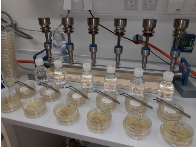
Figure 7: Membrane filtration method for water samples at the water laboratory, Medical University of Graz – Photographer: Sabine Platzer
