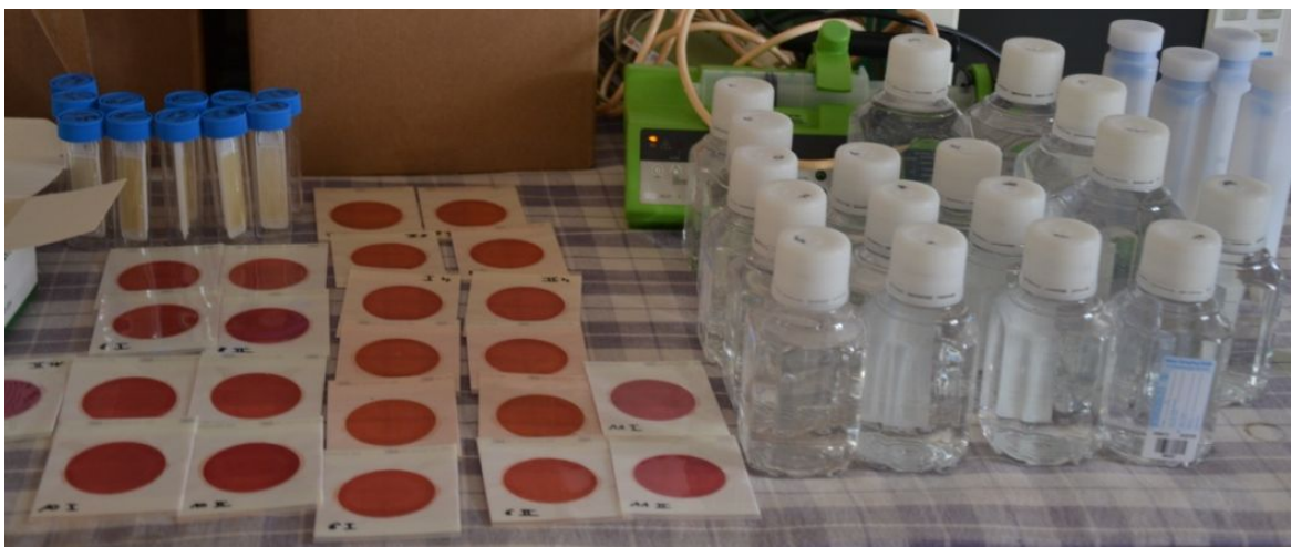
Figure 4: The collected samples: Left front Petrifilms™ behind are the dip slides; right front filled bottles and right behind transport containers filled with the cotton swabs – Photographer: Angelika Schirnhöfer
