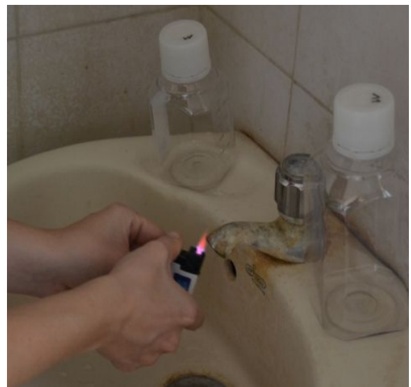
Figure 2: Heating of a water tap, according to the guidelines – Photographer: Angelika Schirnhofner
