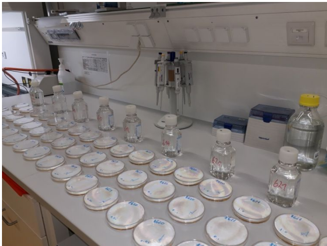
Figure 6: Pour-plate method at the water laboratory, Medical University of Graz – Photographer: Sabine Platzer
