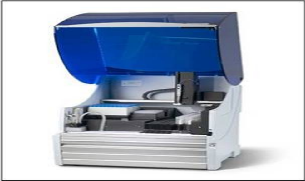
Fig. 32. DS2® Automated ELISA Processing System.
