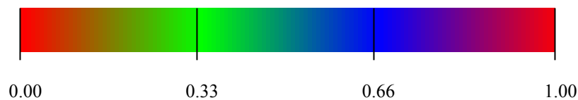
Figure 5: Depiction of hue values assigned to colours in accordance with the system of a colour circle
