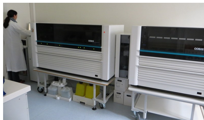
Fig.12: Cobas Ampliprep/Cobas Taq Man for HCV RNA quantitation. The fully automated platform consists of a nucleic acids extraction / PCR mixture preparation device (left) and an amplification / detection device based on the real-time PCR technology.
