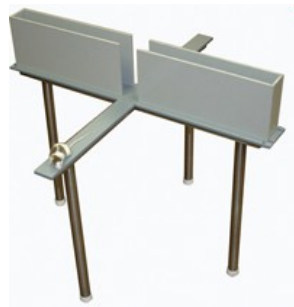
FIGURE 11. Scheme of an Elevated-Plus Maze apparatus. (Taken from: https://www.stoeltingeurope.com/stoelting/2151/2614/1500/EUmaze/Elevated-Plus-Maze )
